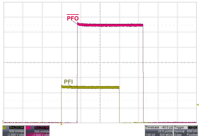
FIGURE 12. ISL705xRH PFI TO PFO RESPONSE
