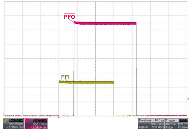
FIGURE 12. ISL705xEH PFI TO PFO RESPONSE
