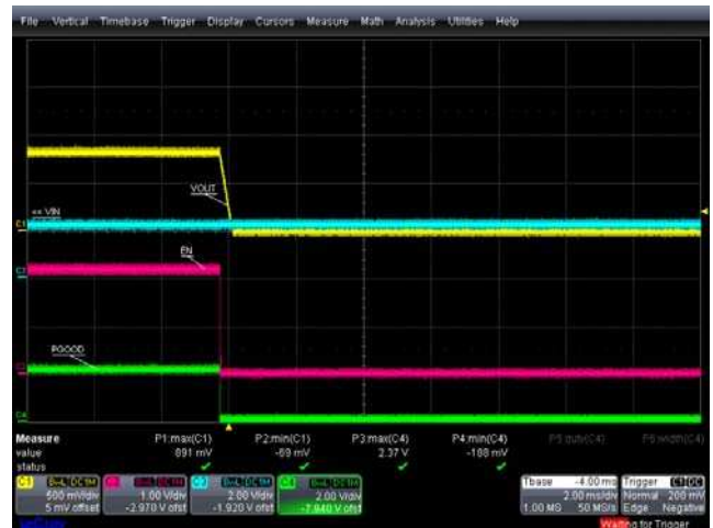
FIGURE 18. POWER-ON AND POWER-OFF, EN = 1 TO 0 , +25^\circ C , V_{IN} = 2.2V , V_{OUT} = 0.8V , I_{OUT} = 0.5A , PGOOD TURN-OFF
