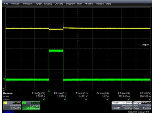
FIGURE 14. TRANSIENT LOAD RESPONSE, V_{IN} = 3.3V , V_{OUT} = 2.5V , C_{OUT} = 220\mu F , 25m\Omega
