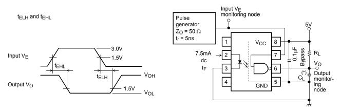
(\*) C<sub>L</sub> is approximately 15pF which includes probe and stray wiring capacitance.
