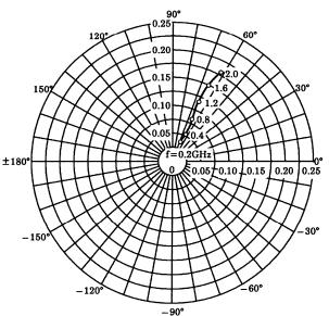
$\begin{array}{l} \text{S}_{22e} \\ \text{V}_{\text{CE}} = 5\text{V} \\ \text{I}_{\text{C}} = 10\text{mA} \\ \text{Ta} = 25^{\circ}\text{C} \\ \text{(UNIT}: \Omega) \end{array}$
