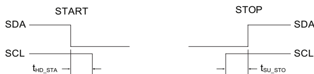
Figure 2: I²C STOP and START Conditions; START: A High "1" to Low "0" Transition on the SDA Line While SCL is High "1" STOP: A Low "0" to High "1" Transition on the SDA Line While SCL is High "1".
