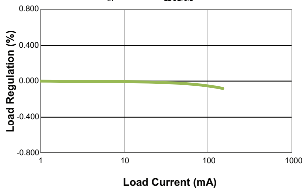
LDOB/C/D Output Voltage Load Regulation ( V_{IN} = 3.6V , V_{LDOB/C/D} = 3.3V )
