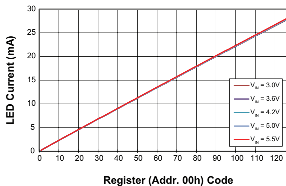
LED Current vs Register (Addr. 00h) Code (4.7μH, 10 WLEDs)
