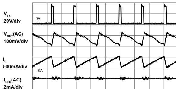
Switching Operation (AAT2893-1, V_{IN} = 3.6V , I_{LED} = 19.8mA , 10 WLEDs)
