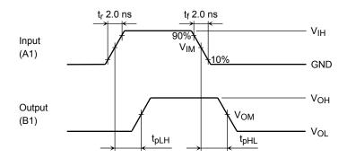
Figure 2 t<sub>pLH</sub>, t<sub>pHL</sub>
