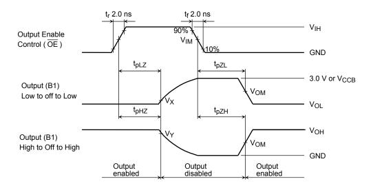
Figure 3  $t_{pLZ}, t_{pHZ}, t_{pZL}, t_{pZH}$
