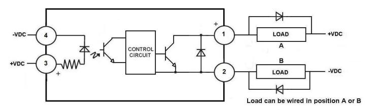
DC Inductive loads must be diode suppressed to prevent damage to SSR
