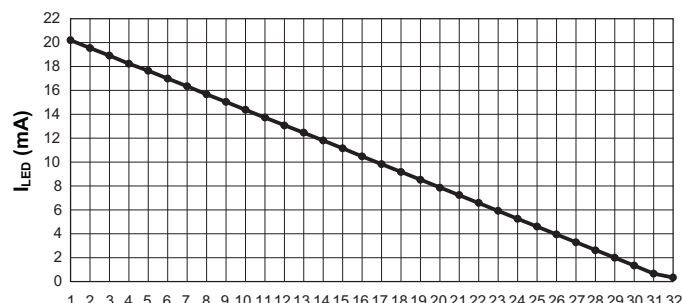
Figure 2: S 2 Cwire Dimming Control at Maximum LED Current (20mA max).
