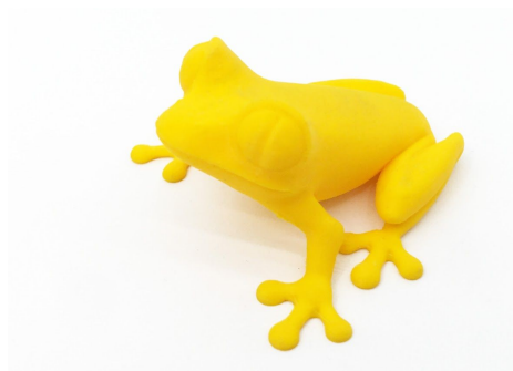
Pict. 20 - 50 microns treefrog is commonly used as a 3D printing benchmark.
