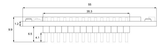
Figure 6 – Mechanical drawing (side view) – Units: mm
