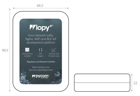
Figure 10 – Mechanical drawing of packaging – Units: mm
