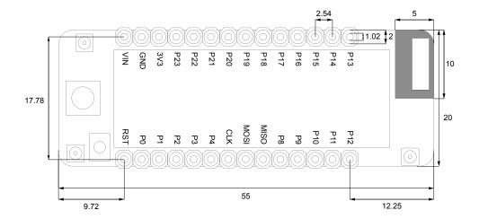
Figure 5 – Mechanical drawing (top down view) – Units: mm
