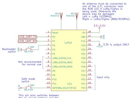
This pin also switches between the on-board antenna and the U.FL connector. For this reason it is not recommended for normal use.
