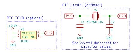
Figure 3 – External RTC crystal circuits
