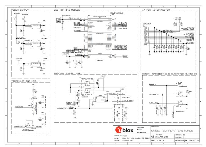
Figure 7: Schematic EVK-F9P-00: GNSS, Antenna supervisor, Supply
