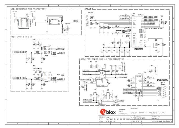
Figure 8: Schematic EVK-F9P-00: Connectors
