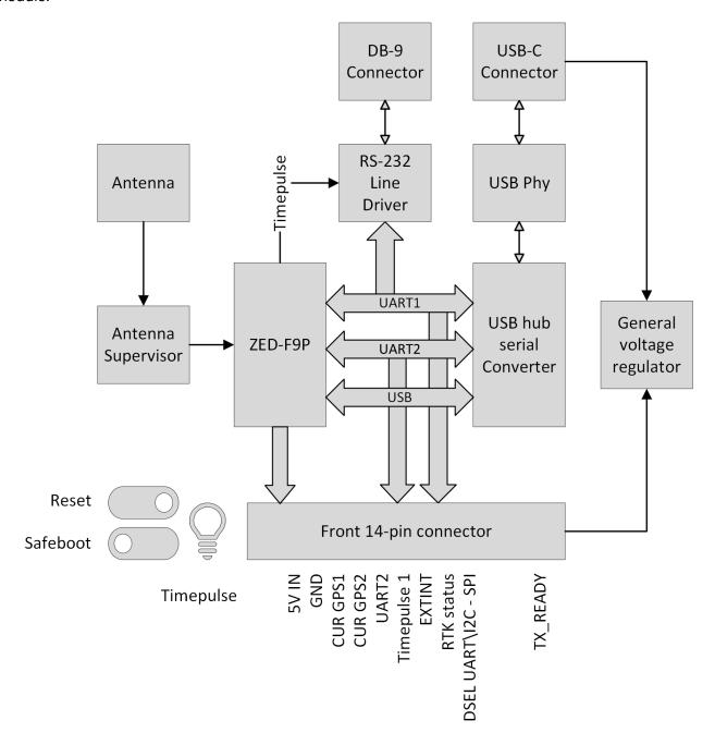
Figure 5: EVB-F9P block diagram
