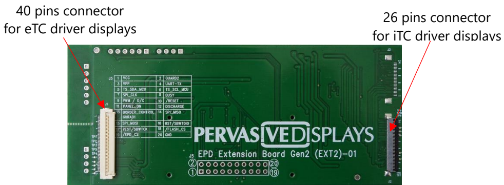
Figure 1-1 EPD Extension Board Gen2 (front view)
