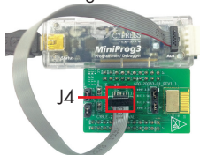
Fig 3: Programming/Debugging with MiniProg3
